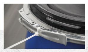
Securing the drums for transport and reuse
